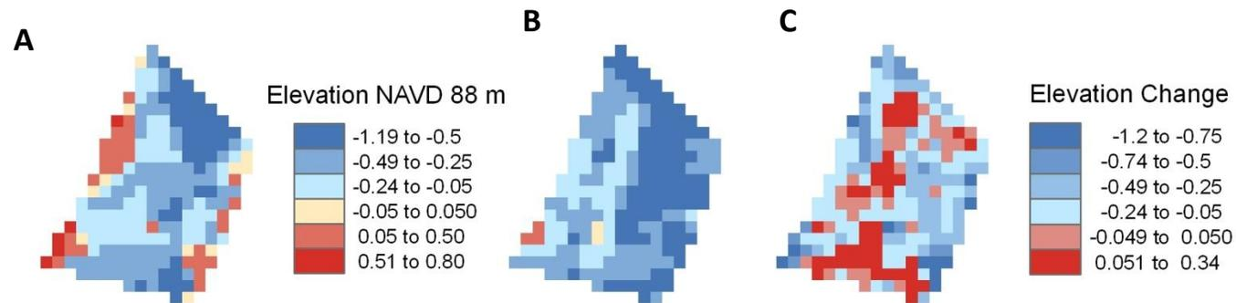
Figure 1.8. Bathymetric maps of elevation (meters NAVD88) of the Central Unit pond breach in 2010 (A), 2011 (B), and the elevation change between years (C).
