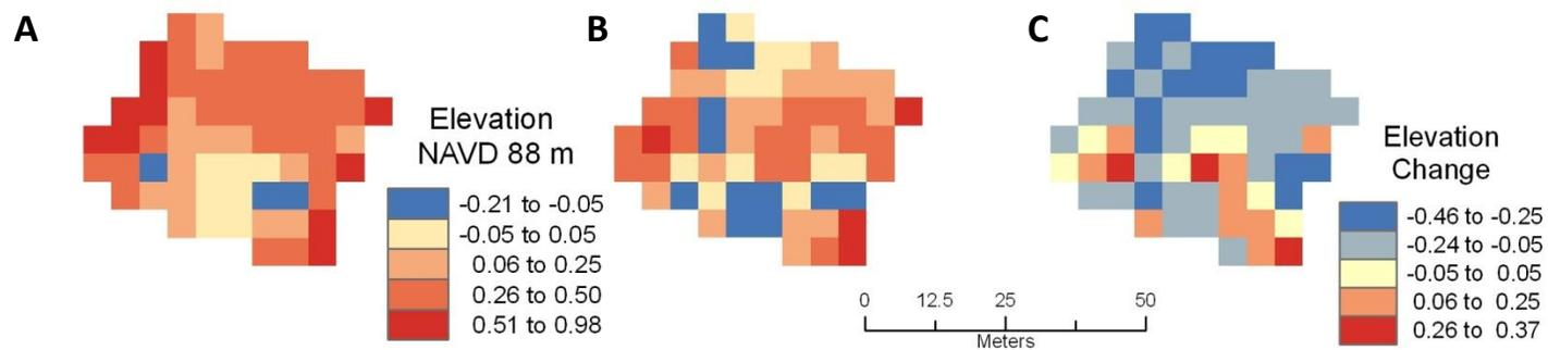
Figure 1.9. Bathymetric maps of elevation (meters NAVD88) of the South Unit salinity reduction breach in 2010 (A), 2011(B), and the elevation change between years (C).
