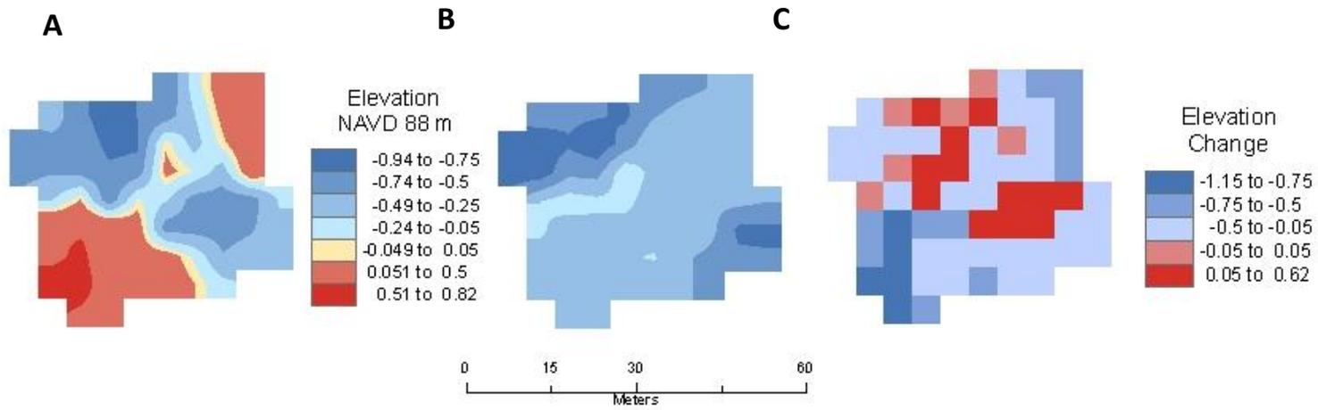
Figure 1.10. Bathymetric maps of elevation (meters NAVD88) of the South Unit northern pond breach in 2011.
