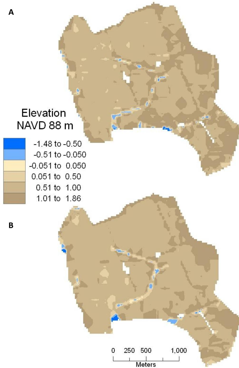
Figure 1.6. Bathymetric map of elevation change (meters NAVD88) of the South Unit between Fall 2010 and Fall 2011. White grid cells indicate no data where islands are present.
