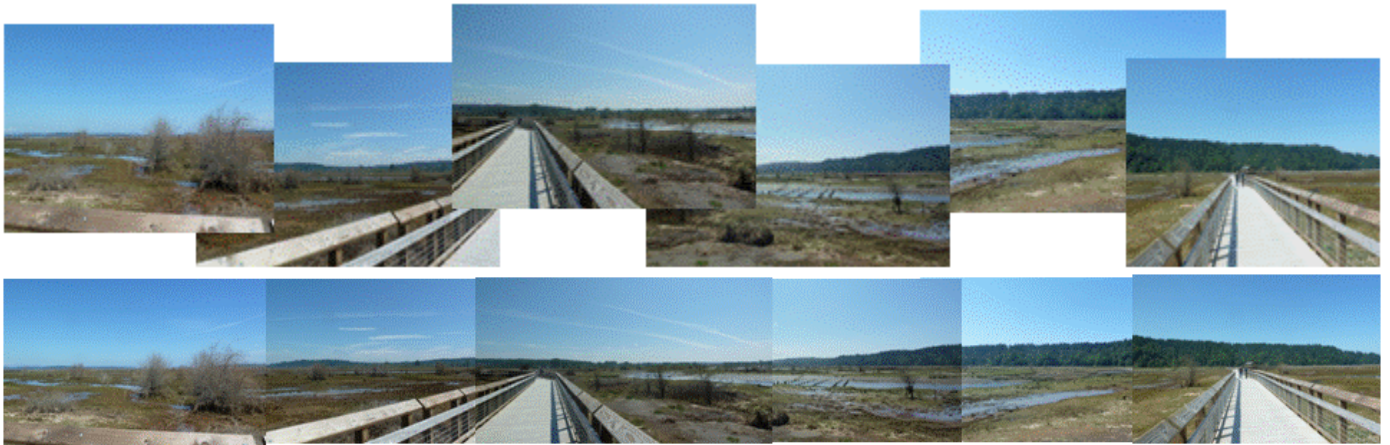
Figure 2. Individual photographs (above) are stitched together to create a 180 or 360 degree panorama (below).
