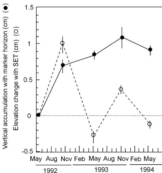
Fig. 1. Three-monthly marker horizon data, showing vertical accumulation, and SET data, showing surface elevation change. Similar data were collected in four marshes simultaneously. Modified from Fig. 4 of Cahoon et al. (1995).
