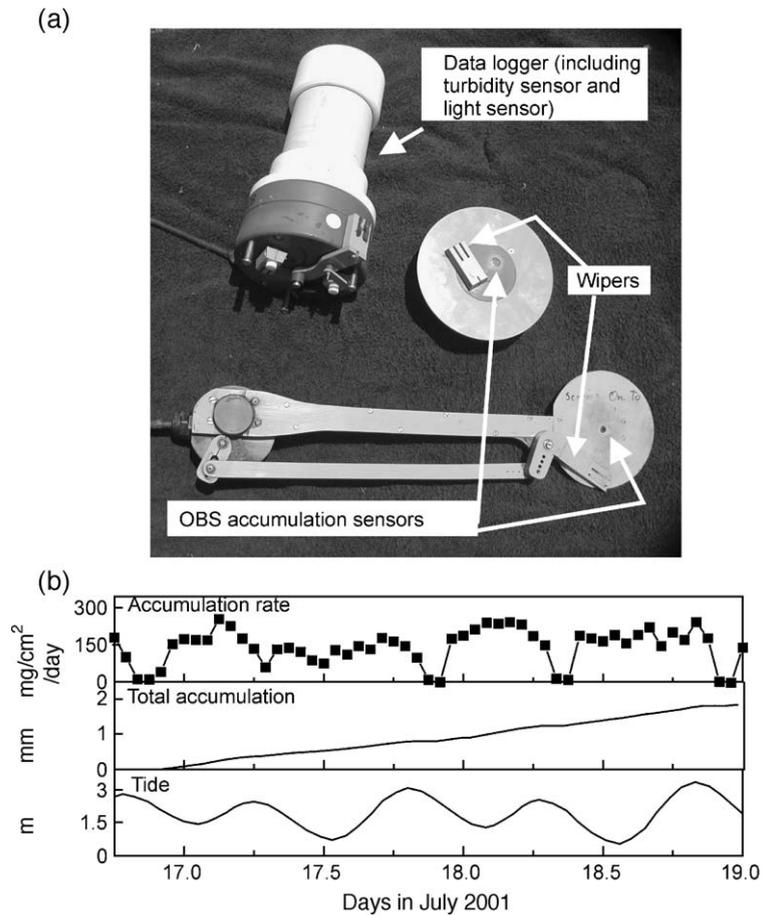
Fig. 5. Hourly accumulation rate obtained with a sediment accumulation sensor (SAS) compared with tidal elevation. This technique allows easy visualisation of total accumulation with both a high temporal and vertical resolution. Modified from Fig. 2 of Thomas et al. (2002).
