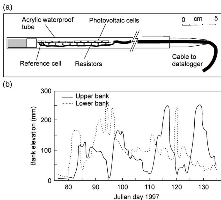
Fig. 11. Photo-electronic erosion pin (PEEP) (a) and corresponding data obtained on an intertidal mudbank (b). Modified from Fig. 1 of Lawler (1991) and from Fig. 3 of Mitchell et al. (1999), respectively.
