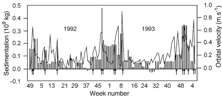
Fig. 9. Weekly amount of accumulated sediment over a given area in a shipping channel deduced from echo-sounder transects, and weekly-average wave orbital velocity at 20 m depth of the one-third highest waves. Modified from Fig. 4 of Verlaan and Spanhoff (2000).
