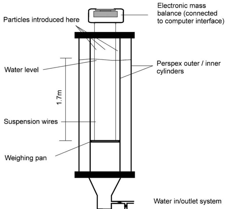
Fig. 6. Fall tower set-up, modified from fig. 2 of Ridd et al. (2001).
