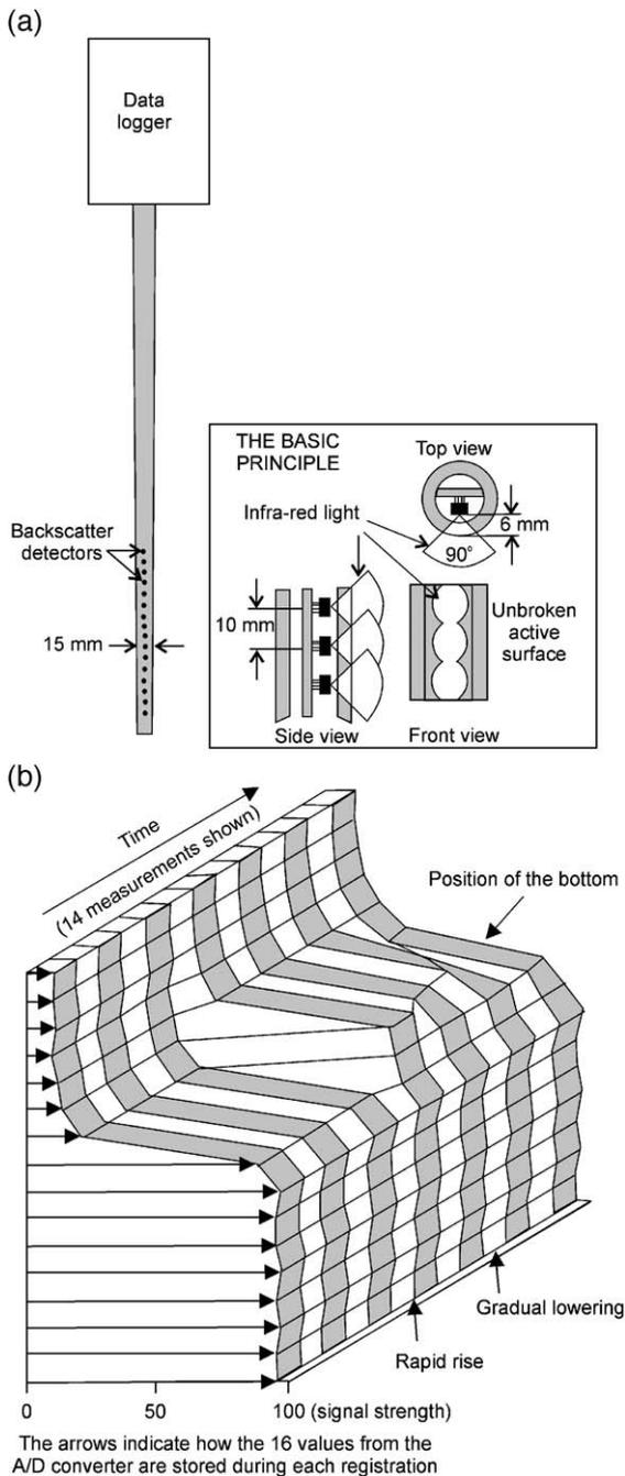
Fig. 10. Sedimeter instrumentation (a) and corresponding data (b). Modified from Figs. 1 and 2 of Erlingsson (1991). The signal strength is indicated as an index value from 0 to 100, and needs to be calibrated in order to transform this index to a precise value of bottom elevation.
