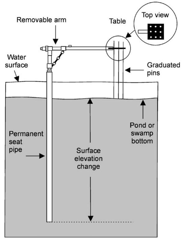
Fig. 8. Sediment elevation table (SET). Modified from Fig. 1 of Cahoon et al. (2002a). Data collected with a SET are shown on Fig. 1.
