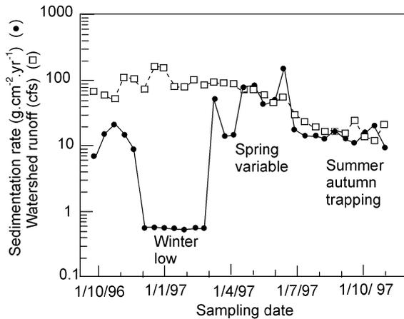
Fig. 2. Two-weekly anchored tile data showing vertical accumulation rates compared with watershed runoff, and revealing no correlation. Modified from Fig. 4 of Pasternack and Brush (2001).
