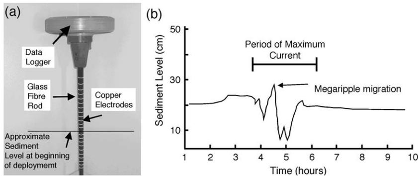
Fig. 12. Electro-resistivity sediment bed level sensor (a) and sand ripples migration measured with the BLS (b) modified from Figs. 1 and 2 of Thomas et al. (2002), respectively.
