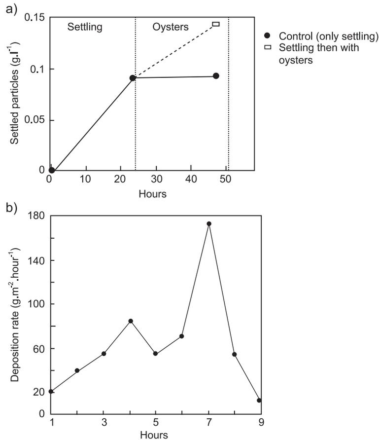
Fig. 4. Accumulation data obtained from SSC changes measurement with samples (a) and self-logging logger (b). Modified from Fig. 3 in Jones et al. (2001) and from Fig. 7 of Halide et al. (2003), respectively.
