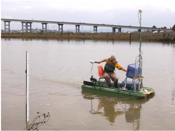
Fig. 2 Field data collection with a shallow-water bathymetry system adjusting bottom elevations to NAVD88 datum by reading an adjacent surveyed staff gage
