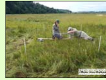
Glenn Guntenspergen and Kelley Turner using Surface Elevation Table to measure elevation changes.
