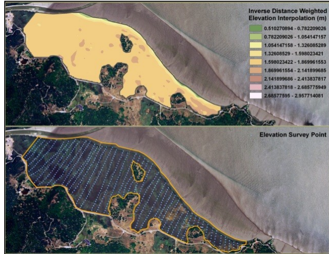
Figure 1. RTK GPS elevation survey points (bottom) and interpolated digital elevation model (DEM; top).
